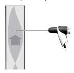
➤ Align the flue gas probe in the flue gas duct so that the tip is in the centre of the flow (area of the highest flue gas temperature).
