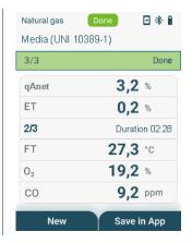
Remove flue gas probe from the flue gas duct and purge with fresh air.
