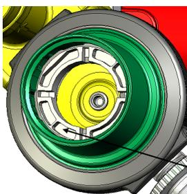
1. Remove the OPSO cap and adjust to give the desired pressure.
