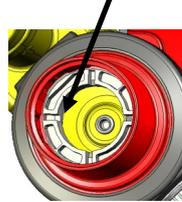
Please note that OPSO settings will not adjust with outlet pressures, so OPSO settings should be considered when adjusting the outlet pressure.
