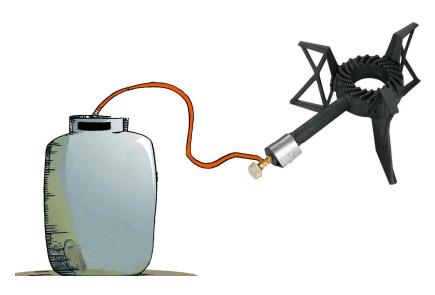
Be very careful when you use this stove under 0°C. When the temperature is under 0°C, the rubber joints may harden and cause a gas leak.
